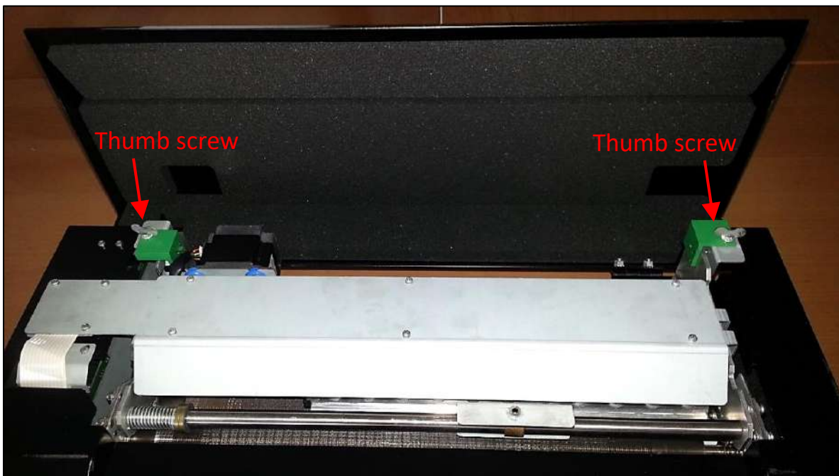
Shows paper cleanout under top housing lid
